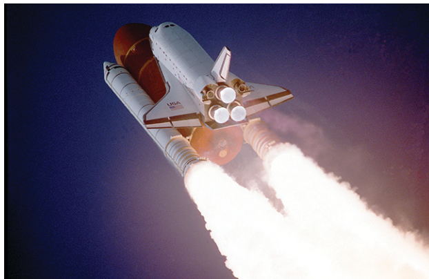
Figure 18.28 Before the fleet's retirement in 2011, liquid hydrogen and liquid oxygen were used in the three main engines of a space shuttle. Two compartments in the large tank held these liquids until the shuttle was launched. (credit: "reynnermedia"/Flickr)
