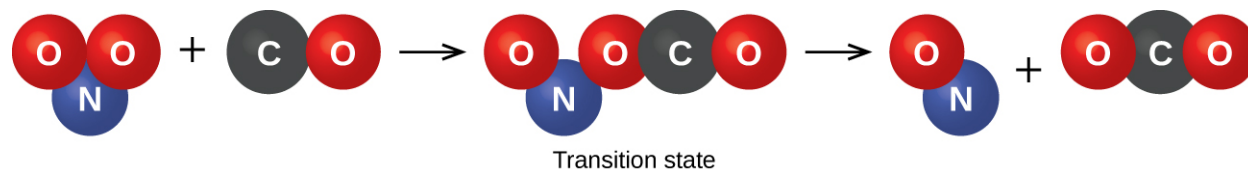
Figure 17.17 The probable mechanism for the reaction between \text{NO}_2 and \text{CO} to yield \text{NO} and \text{CO}_2 .
