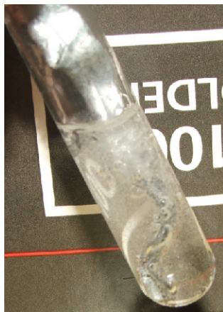
Figure 18.7 Zinc is an active metal. It dissolves in hydrochloric acid, forming a solution of colorless \text{Zn}^{2+} ions, \text{Cl}^- ions, and hydrogen gas.
