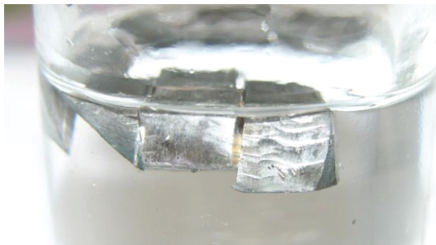
Figure 18.3 Lithium floats in paraffin oil because its density is less than the density of paraffin oil.
