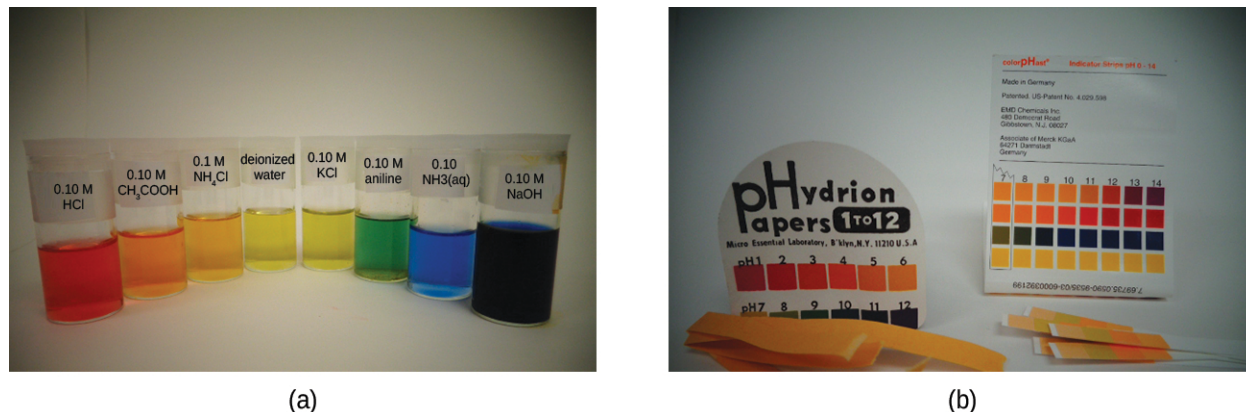
Figure 14.5 (a) A solution containing a dye mixture, called universal indicator, takes on different colors depending upon its pH. (b) Convenient test strips, called pH paper, contain embedded indicator dyes that yield pH-dependent color changes on contact with aqueous solutions. (credit: modification of work by Sahar Atwa)
