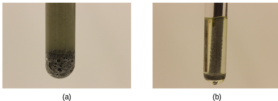
Figure 17.6 (a) Iron powder reacts rapidly with dilute hydrochloric acid and produces bubbles of hydrogen gas: 2\text{Fe}(s) + 6\text{HCl}(aq) \longrightarrow 2\text{FeCl}_3(aq) + 3\text{H}_2(g) . (b) An iron nail reacts more slowly because the surface area exposed to the acid is much less.
