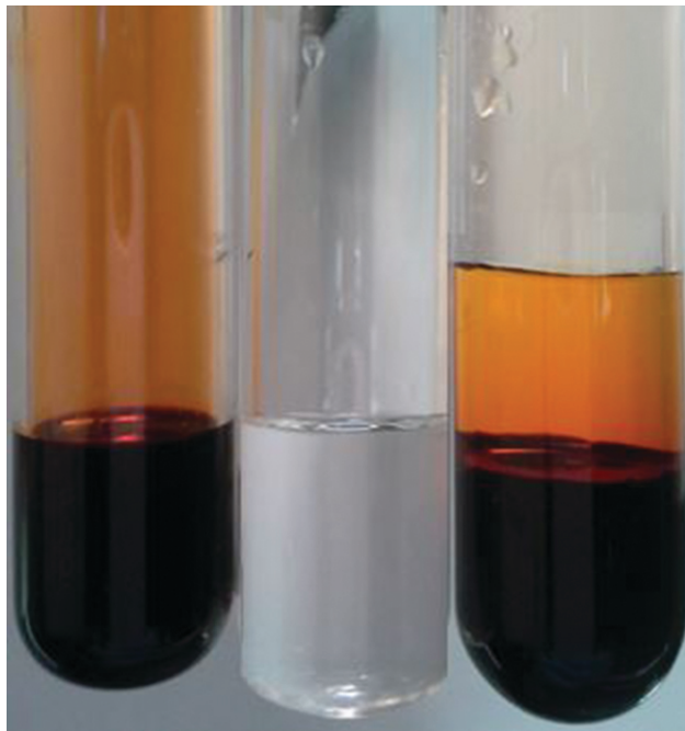
Figure 11.15 Bromine (the deep orange liquid on the left) and water (the clear liquid in the middle) are partially miscible. The top layer in the mixture on the right is a saturated solution of bromine in water; the bottom layer is a saturated solution of water in bromine. (credit: Paul Flowers)
