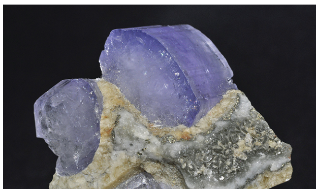
Figure 15.8 Crystal of the mineral hydroxyapatite, \text{Ca}_5(\text{PO}_4)_3\text{OH} , is shown here. The pure compound is white, but like many other minerals, this sample is colored because of the presence of impurities.
