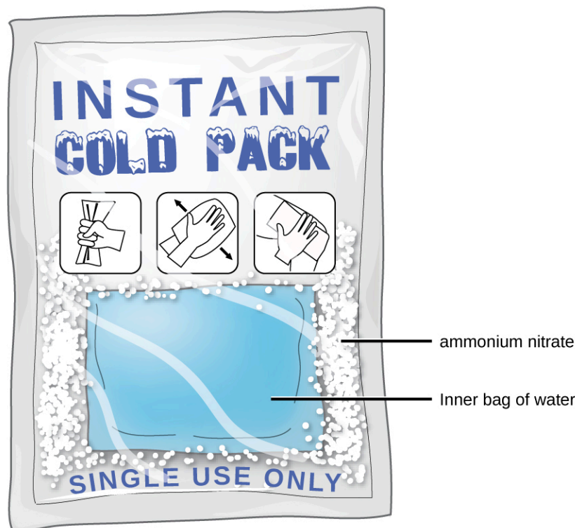
Figure 11.5 An instant cold pack gets cold when certain salts, such as ammonium nitrate, dissolve in water—an endothermic process.
