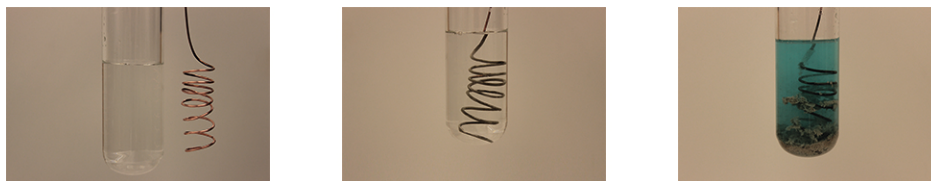
Figure 16.2 A copper wire and an aqueous solution of silver nitrate (left) are brought into contact (center) and a spontaneous transfer of electrons occurs, creating blue \text{Cu}^{2+}(aq) and gray \text{Ag}(s) (right).
