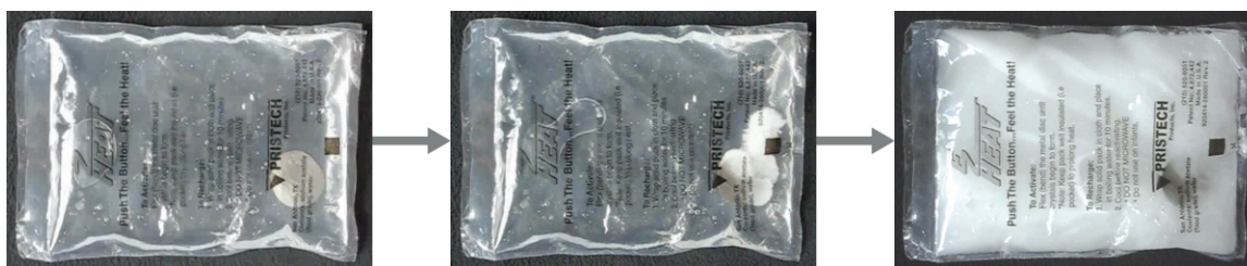
Figure 11.17 This hand warmer produces heat when the sodium acetate in a supersaturated solution precipitates. Precipitation of the solute is initiated by a mechanical shockwave generated when the flexible metal disk within the solution is “clicked.” (credit: modification of work by “Velega”/Wikimedia Commons)
