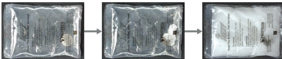
Figure 9.15 Chemical hand warmers produce heat that warms your hand on a cold day. In this one, you can see the metal disc that initiates the exothermic precipitation reaction. (credit: modification of work by Science Buddies TV/YouTube)
