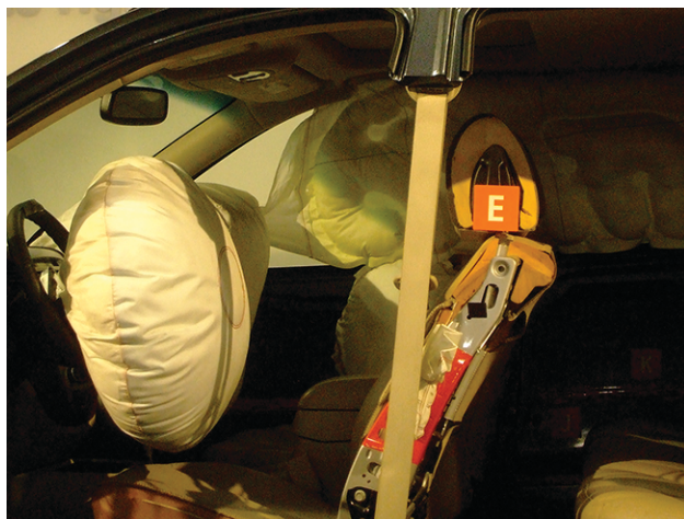
Figure 7.12 Airbags deploy upon impact to minimize serious injuries to passengers. (credit: Jon Seidman)
