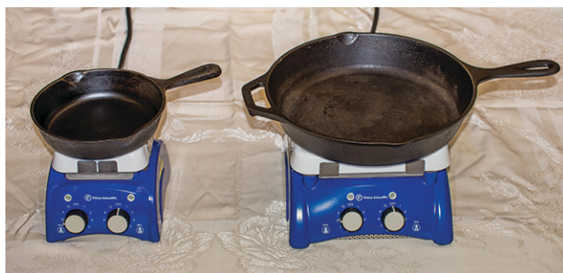
Figure 9.8 Because of its larger mass, a large frying pan has a larger heat capacity than a small frying pan. Because they are made of the same material, both frying pans have the same specific heat. (credit: Mark Blaser)
