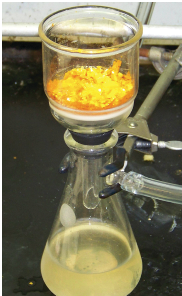
Figure 7.17 Precipitate may be removed from a reaction mixture by filtration.
