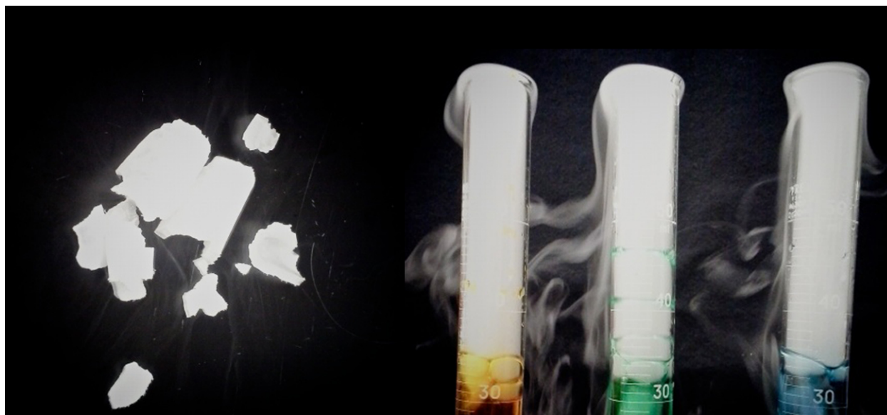
Figure 10.1 Solid carbon dioxide (“dry ice”, left) sublimates vigorously when placed in a liquid (right), cooling the liquid and generating a dense mist of water above the cylinder. (credit: modification of work by Paul Flowers)
