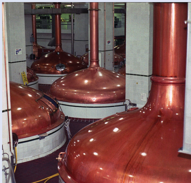
Figure 6.7 An oxide of carbon is removed from these fermentation tanks through the large copper pipes at the top. (credit: "Dual Freq"/Wikimedia Commons)
