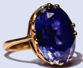
Figure 3.42 Although pure aluminum oxide is colorless, trace amounts of iron and titanium give blue sapphire its characteristic color. (credit: modification of work by Stanislav Doronenko)
